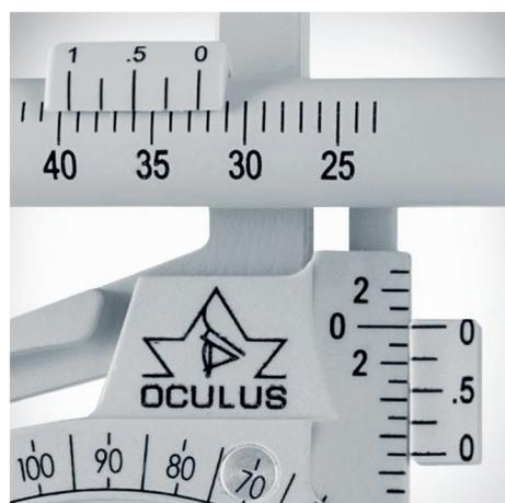
Settings with vernier scale accurate to 0.25 mm (0.01 in)
